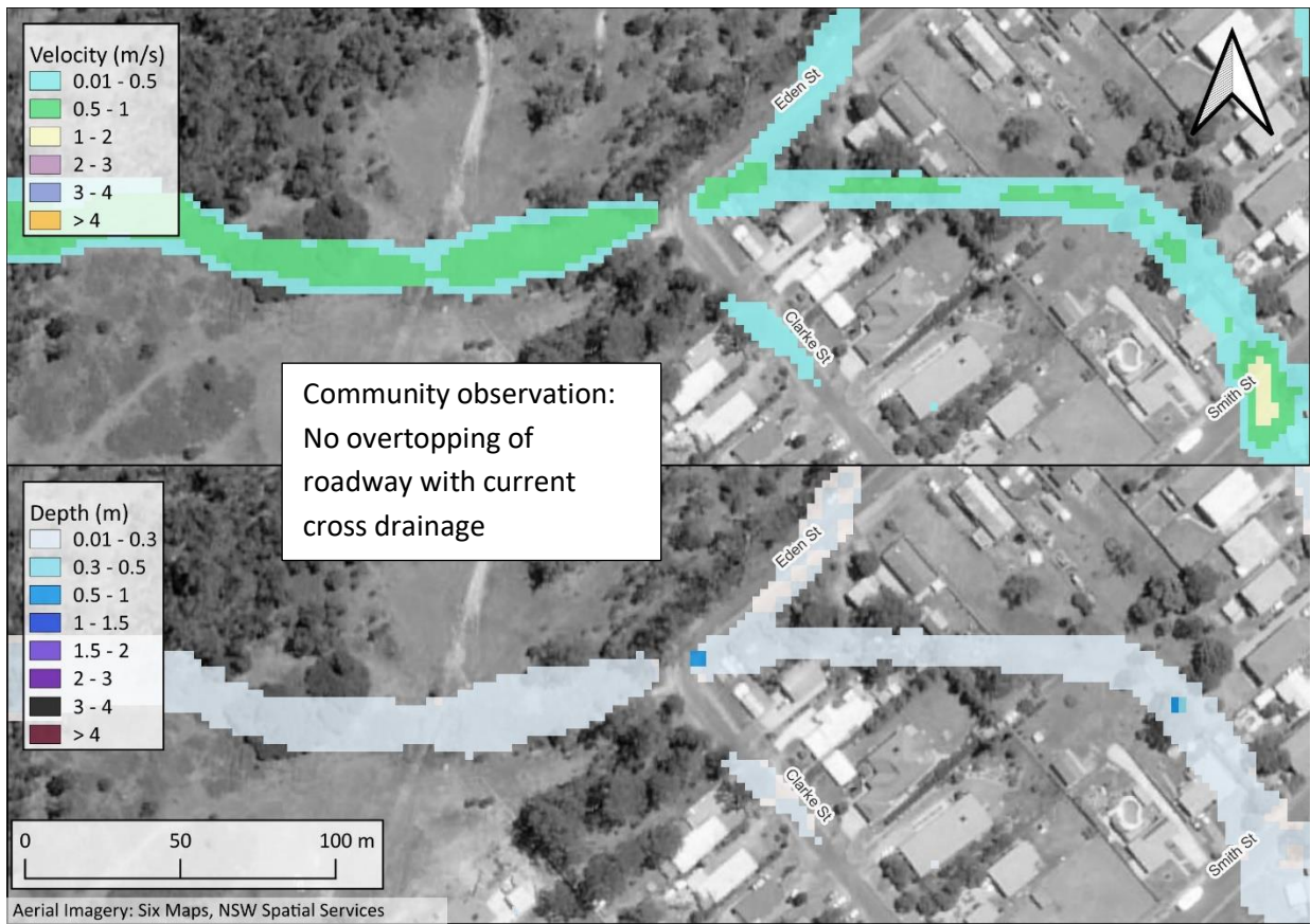
Figure 4-7 20% AEP Flood Behaviour at Eden Street and Clarke Street
